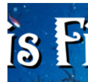
If text is part of a bitmap image, the pixels determine smoothness.
